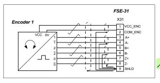
**Note**: This figure applies to the FSE-31 module revision F or later. Make sure you connect the safety encoder according to this figure. You can see the revision of the module in the type designation label (see page 15).
