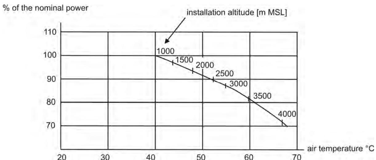
Check the air temperature and the installation altitude separately. Should there be differing air temperatures and installation altitudes concurrently, the factors concerning available nominal power need to be multiplied.
