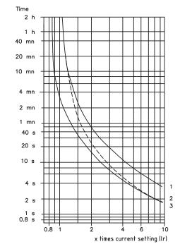
1 —— Balanced operation, 3-phase, from cold state.
