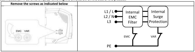
The Optidrive product range has input supply voltage surge suppression components fitted to protect the drive from line voltage transients, typically originating from lightning strikes or switching of high power equipment on the same supply.
