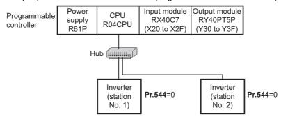
Network parameter setting of the master station Network parameters are set as below.
