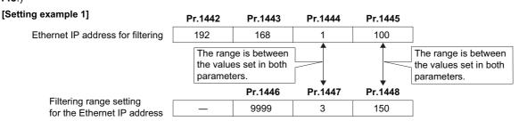
In this case, the IP address range in which Ethernet communication is permitted is "192.168.x (1 to 3).xxx (100 to 150)".
