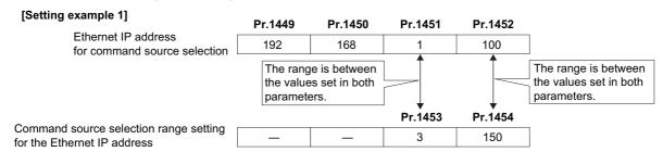
In this case, the IP address range for command source selection via Ethernet communication is "192.168.x (1 to 3).xxx (100 to 150)".
