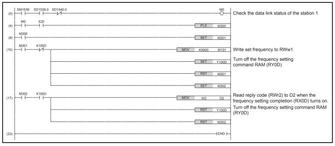
To continuously change the running frequency from the programmable controller
