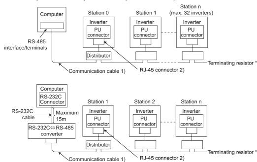
\* The inverters may be affected by reflection depending on the transmission speed or transmission distance. If this reflection hinders communication, provide a terminating resistor. If the PU connector is used to make a connection, use a distributor since a terminating resistor cannot be fitted. Connect the terminating resistor to only the inverter remotest from the computer. (Terminating resistor: 100Ω)
