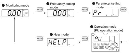
If  $\[PU\]$  cannot be displayed by pressing the  $\[Alpha\]$  /  $\[V\]$  key in the External operation mode  $\[Black]$  ( $\[Pr. 79\]$  operation mode selection  $\[Pr. 79\]$  operation mode selection.
