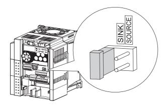
The input signals are set to sink logic (SINK) when shipped from the factory.
