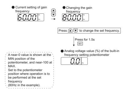
Method to adjust any point by turning the built-in frequency setting potentiometer. (application of 5V)
