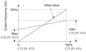
Frequency setting signal (Built-in frequency setting potentiometer)
