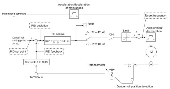
\*1 The main speed can be selected from all operation mode such as external (analog voltage input, multi-speed), PU (digital frequency setting), and communication (RS-485).
