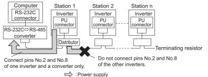
• Do not connect the PU connector to the computer's LAN board, FAX modem socket or telephone modular connector. The product could be damaged due to differences in electrical specifications.
