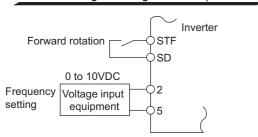
Connection diagram using terminal 2 (0 to 10VDC)
