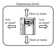
When using the inverters at the surrounding air temperature of 40℃ or less, the inverters can be installed without any clearance between them (0cm clearance).
