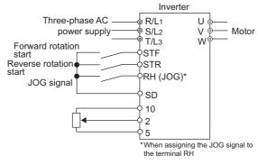
Connection diagram for external Jog operation
