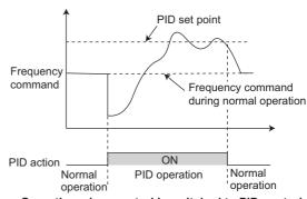
Operation when control is switched to PID control during normal operation
