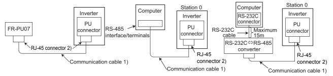
● Combination of computer and multiple inverters (1:n connection)
