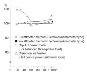
Example of Measuring Inverter Output Power
