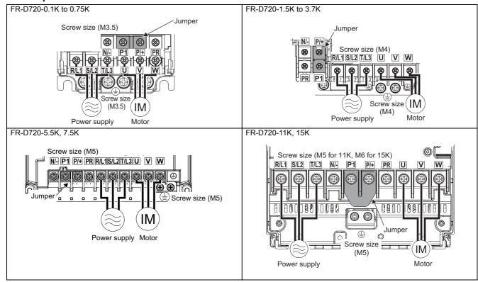
\* For wiring to earth (ground) terminals of FR-D720-5.5K and 7.5K, use the earthing cable wiring space (marked with an arrow) to route the wires.
