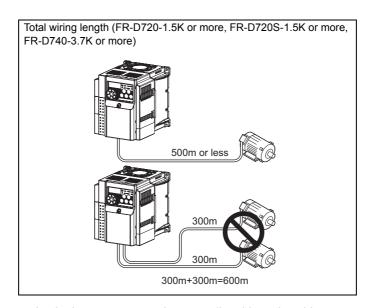
When driving a 400V class motor by the inverter, surge voltages attributable to the wiring constants may occur at the motor terminals, deteriorating the insulation of the motor. (Refer to page 84)
