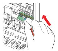
When using a single wire or a stranded wire without a blade terminal, push an open/close button all the way down with a flathead screw driver, and insert the wire.
