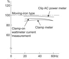
Example of measuring inverter input current
