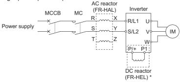
When connecting the FR-HEL, remove the jumper across terminals P/+ and P1. The wiring length between the FR-HEL and inverter should be 5m maximum and minimized.
