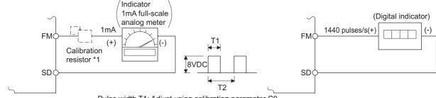
Pulse width T1: Adjust using calibration parameter C0 Pulse cycle T2: Set with Pr. 55 (frequency monitor) Set with Pr. 56 (current monitor)
