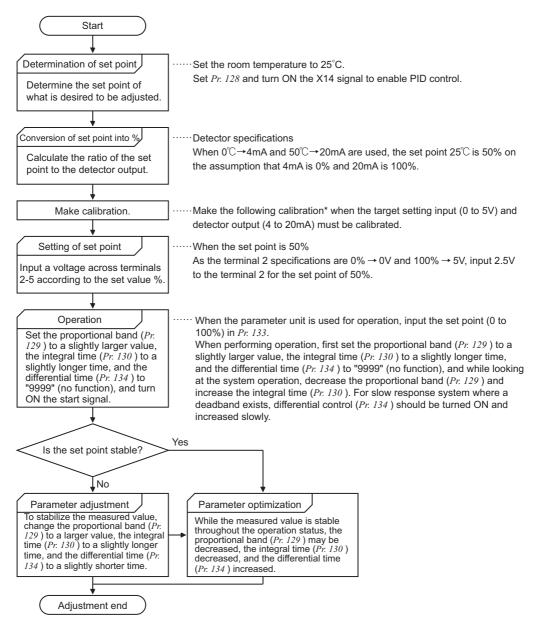
\*When calibration → Using calibration *Pr. 902* and *Pr. 903* (terminal 2) or *Pr. 904* and *Pr. 905* (terminal is required 4), calibrate the detector output and target setting input.
