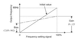
•When ratio ( $Pr.\ 128$  = "42, 43") is selected for addition method, PID control × (ratio of main speed) is added to the main speed. The ratio is determined by the  $Pr.\ 125$  Terminal 2 frequency setting gain frequency and C2 ( $Pr.\ 902$ ) Terminal 2 frequency setting bias frequency. The frequency setting signal is set to 0 to 60Hz in the range between 0 to 100% in the initial setting. The ratio is (×100%) when the main speed is 60Hz and (×50%) when 30Hz.
