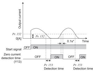
The zero current detection signal (Y13) holds the signal for approximately 0.1s once turned ON.
