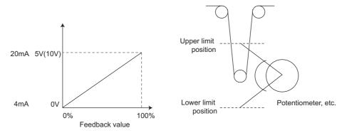
(Example) Control at a dancer center position using a 0 to 7V potentiometer
