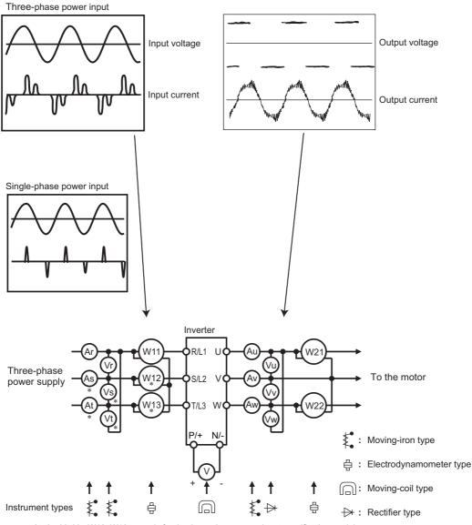
\* At, As, Vt, Vs, W12, W13 are only for the three-phase power input specification models.
