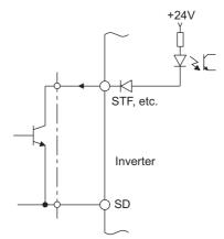
External signal input using transistor
