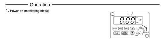
2. Make sure that the inverter is in PU mode with MODE key.
