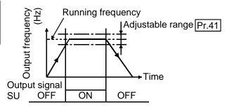
• Use any of Pr. 190 to Pr. 192 to allocate the terminal used for SU signal output. Refer to page 150 for Pr. 190 to Pr. 192 (output terminal function selection).
