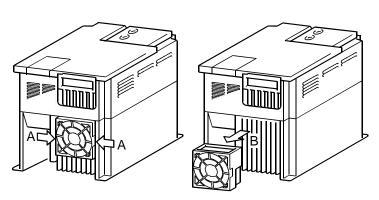
4) Remove the cooling fan and cooing fan cover.
