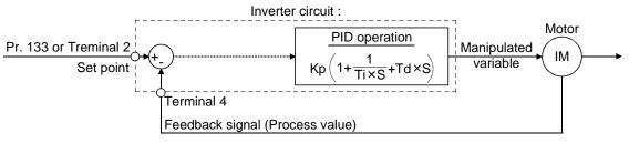
Kp: Proportion constant Ti: Integral time S: Operator Td: Differential time
