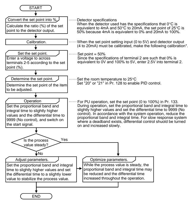
\* When calibration is required, use Pr. 902 and Pr. 903 (terminal 2) or Pr. 904 and Pr. 905 (terminal 4) to calibrate the detector output and set point setting input in the PU mode during an inverter stop.
