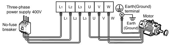
The power supply cables must be connected to L<sub>1</sub>, L<sub>2</sub>, L<sub>3</sub>. If they are connected to U, V, W, the inverter will be damaged.
