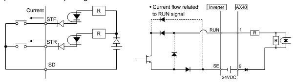
When using an external power supply for transistor output, use terminal PC as a common to prevent misoperation caused by undesirable current.
