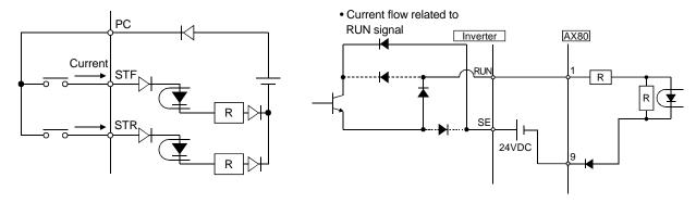
When using an external power supply for transistor output, use terminal SD as a common to prevent misoperation caused by undesirable current.
