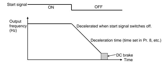
(2) Pr. 250 = 0 to 100 seconds (output is shut off after preset time)
