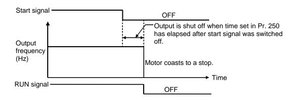
When the Pr. 250 value is 8888, the functions of terminals STF and STR change as shown below:
