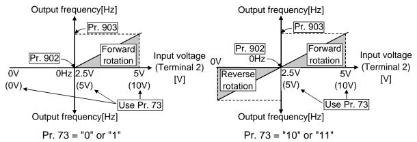
When Pr.73 = "10" as factory-set, Pr.902 = 2.5V. When Pr.73 = "11", Pr.902 = 5V.
