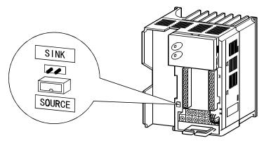
Note: 1. Make sure that the front cover has been installed securely.
