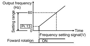
Note: The inverter will not start if the frequency setting signal is less than the value set in Pr. 13 "starting frequency".
