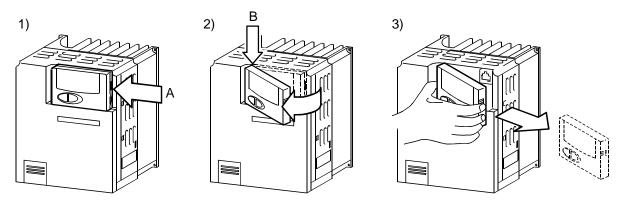
(If the above procedure is not used for removal, the internal connector may be damaged by the force applied.)
