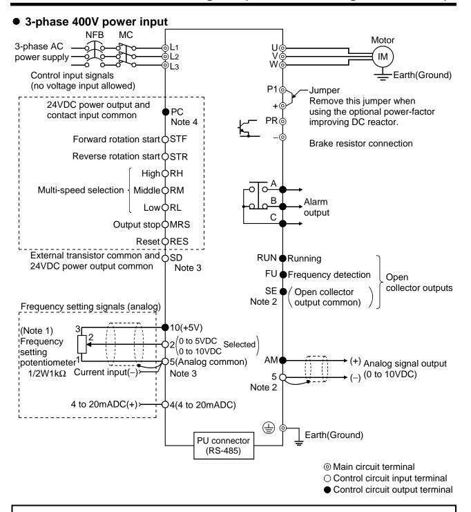
Note: 1. If the potentiometer is to be operated often, use a  $2W1k\Omega$  potentiometer.
