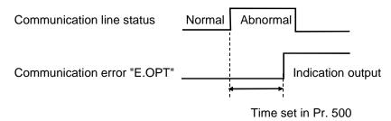
If a communication line fault still persists after the time set in Pr. 500 has elapsed, it is recognized as a communication error and the communication error indication "E.OPT" is output.
