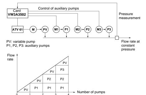
The Altivar 61 controls the pumps via logic outputs LO51, LO52, LO53, etc., according to the operating mode that has been programmed.
