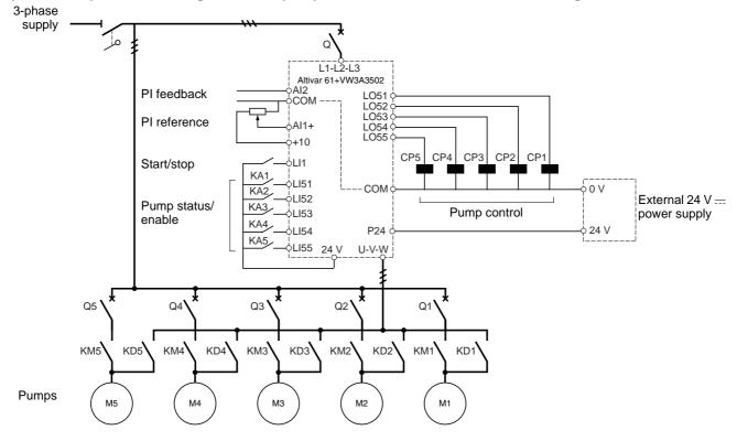
Each pump is controlled by a logic output.
