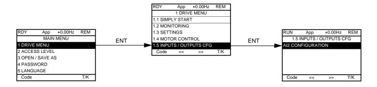
Configure AI2 according to the pressure sensor being used (Example: 4 - 20 mA)
