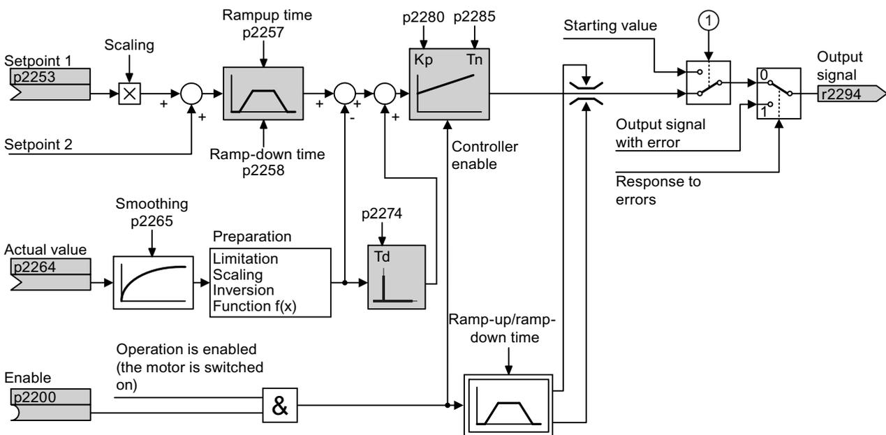
Figure 8-32 Simplified representation of the technology controller
