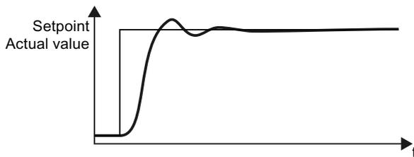
**Optimum controller behavior for fast correction and quick compensation of noise components.**
