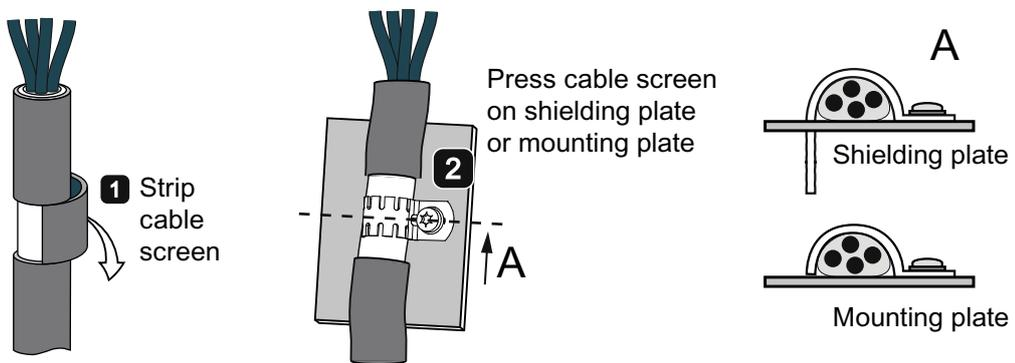
Figure 3-4 Shield connection - detail
