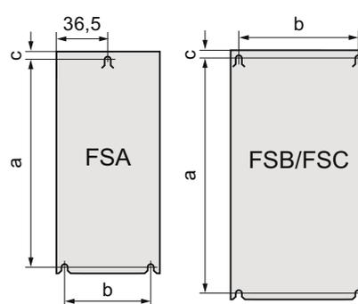
Drilling patterns for PM230, PM240-2, FSA ... FSC
