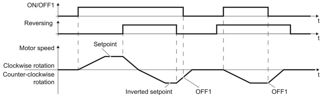
Figure 8-3 Two-wire control, method 1
