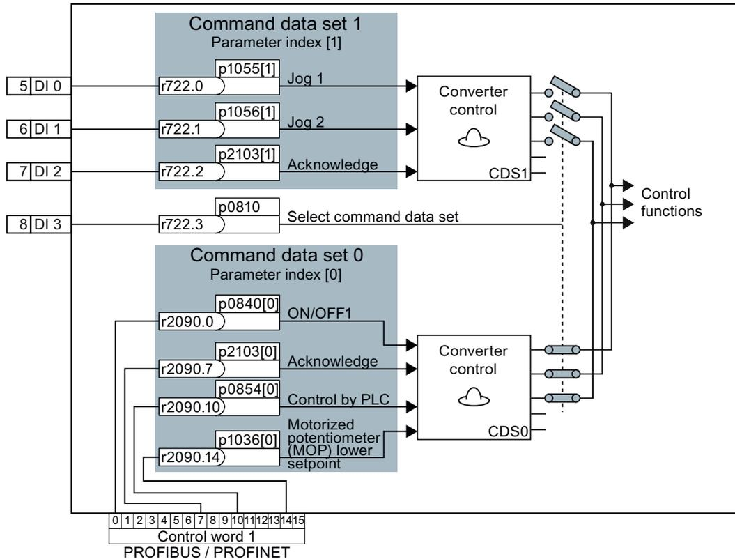
Figure 8-10 Example for the various command data sets
