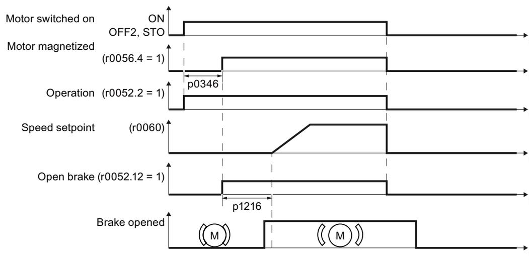
Figure 8-28 Controlling the motor holding brake after an OFF2 command or STO
