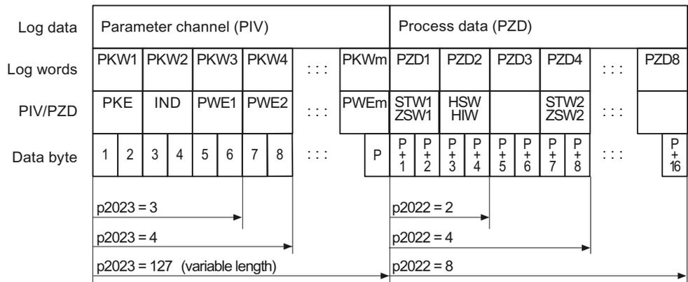
Figure 7-9 USS telegram - user data structure
