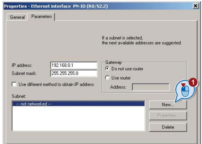
Use the "New" button (①) to either create a new PROFINET subnet or select an existing one.
