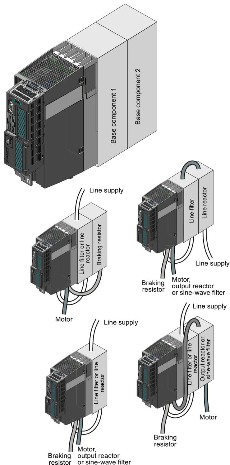
Figure 3-1 Base components and wiring options
