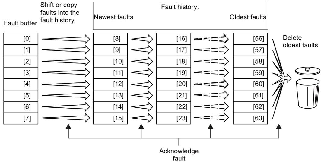
Figure 11-8 Fault history after acknowledging the faults
