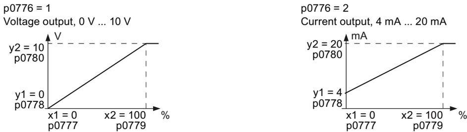
Figure 6-4 Examples for scaling characteristics
