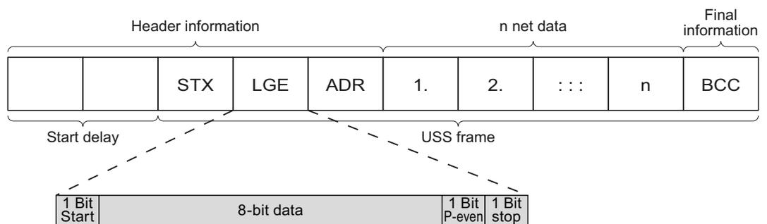
Figure 7-8 Structure of a USS telegram
