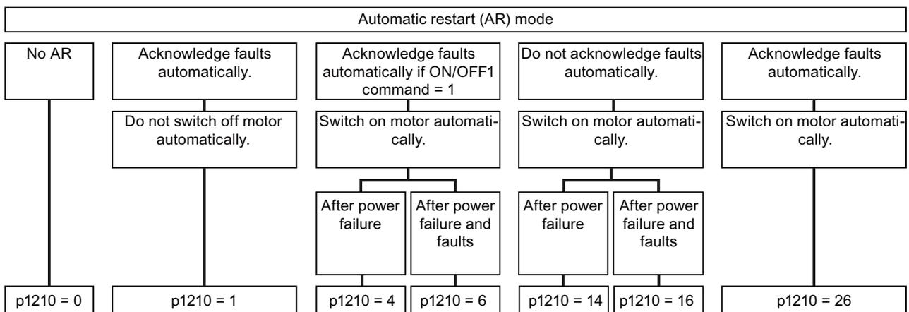
Figure 8-29 Selecting the automatic restart mode
