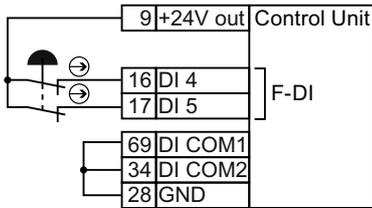
Figure A-9 Connecting a sensor, e.g. Emergency Stop mushroom pushbutton or limit switch
