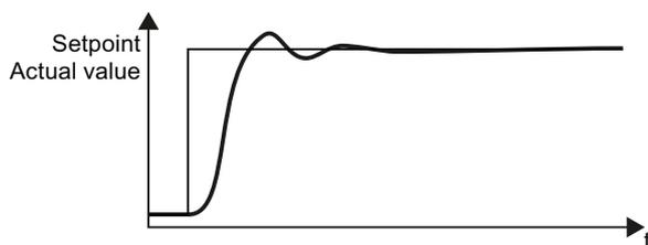
**Optimum control behavior for fast correction and quick compensation of noise components.**
