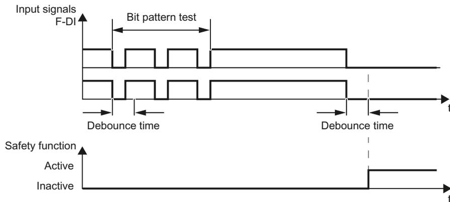
Figure 8-37 Filter for suppressing temporary signal changes
