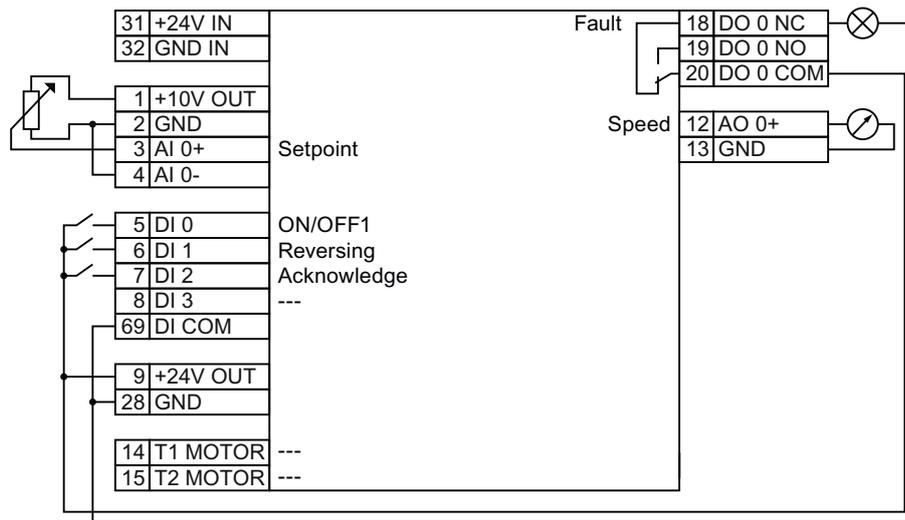
Figure 5-2 Wiring example to use the factory settings
