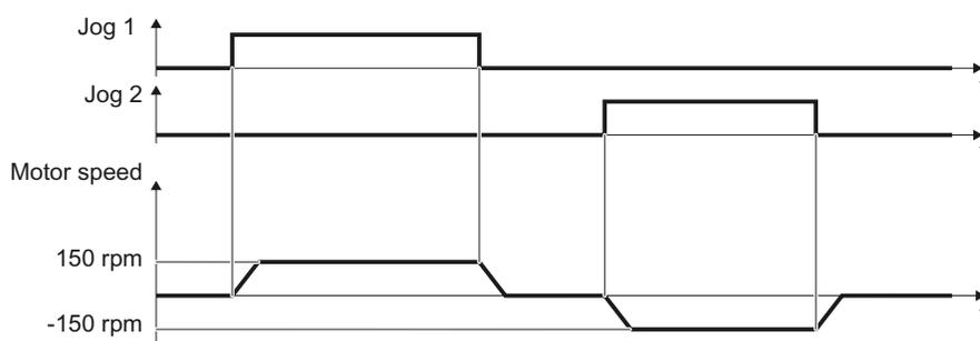
Figure 5-7 Jogging the motor in the factory setting
