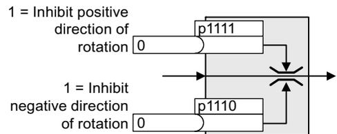
Table 8- 26 Examples of settings to inhibit the direction of rotation
