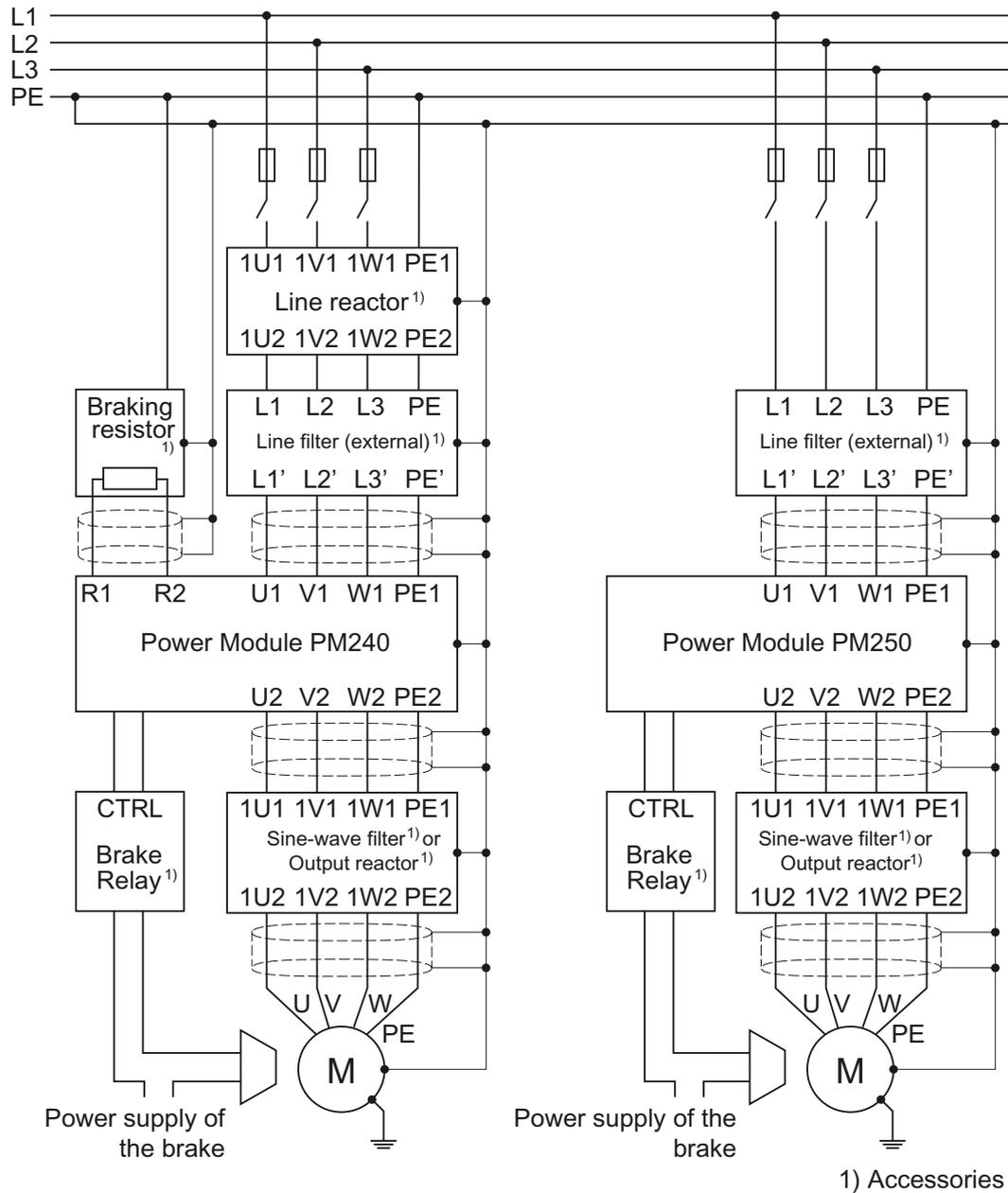
Figure 3-2 Connections for PM240 and PM250 Power Modules
