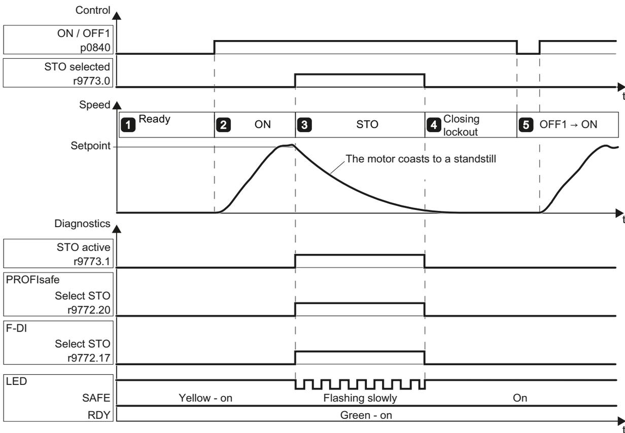
Figure 8-41 STO acceptance test for basic functions
