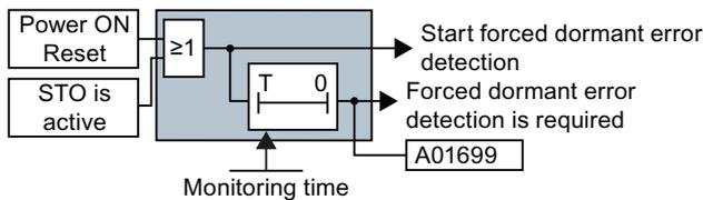
Figure 8-38 Triggering and monitoring the forced checking procedure
