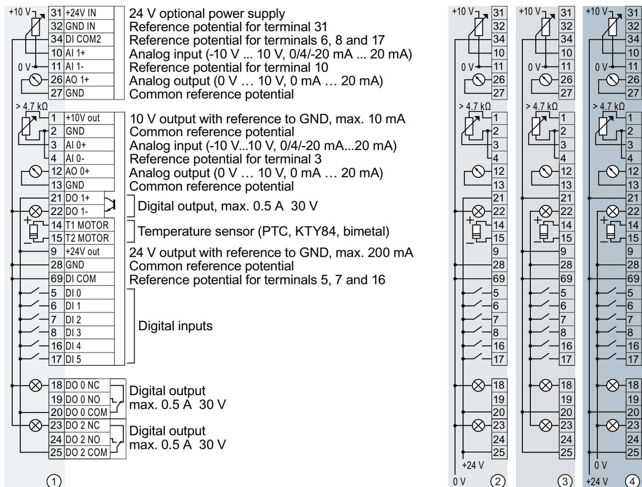
You may use the internal 10V power supply or an external voltage source for the analog input.
