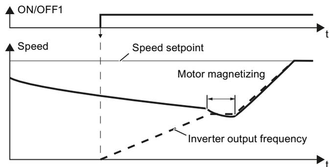
Principle of operation of the "flying restart" function
