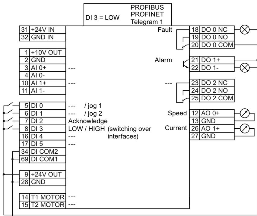
Figure 5-5 Wiring example to use the factory settings
