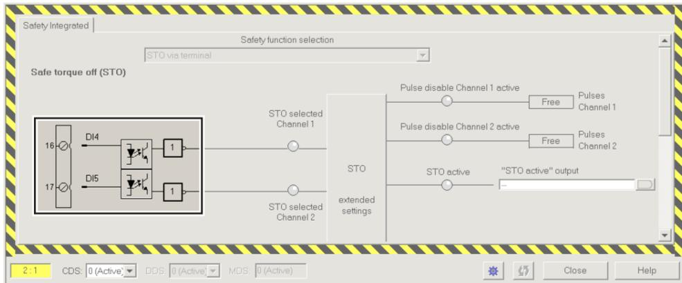
Figure 8-39 Example: automatic assignment of digital inputs DI 4 and DI 5 with STO
