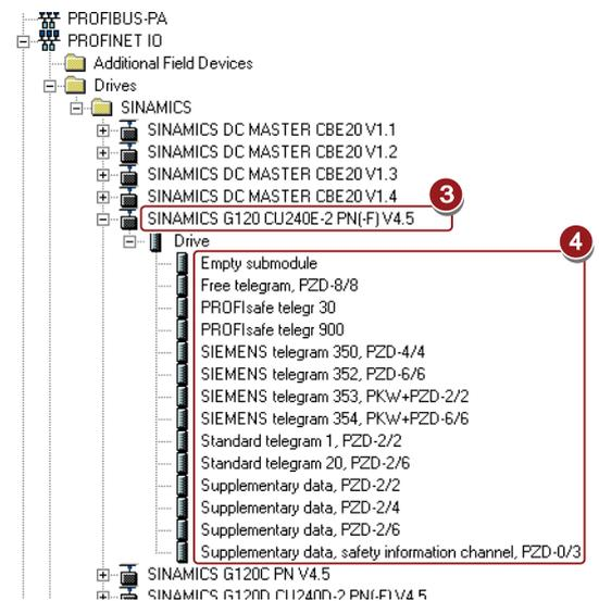
Then save your hardware configuration with "Save and compile" (
