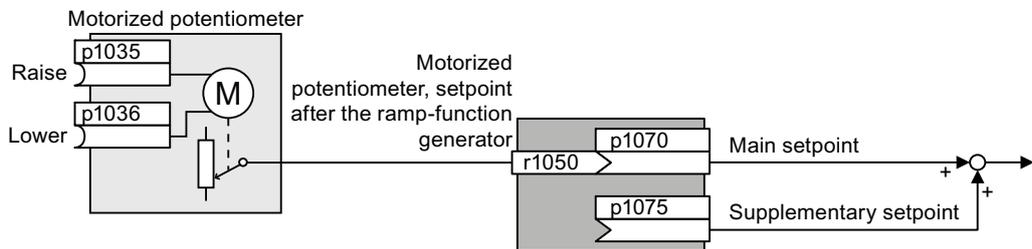
Figure 8-14 Motorized potentiometer as setpoint source
