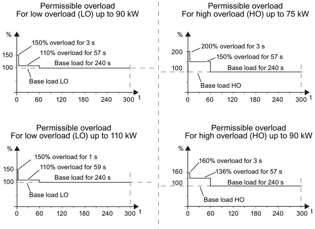
Figure 12-1 Duty cycles, "High Overload" and "Low Overload"
