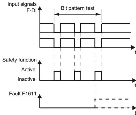
Figure 8-36 Converter response to a bit pattern test
