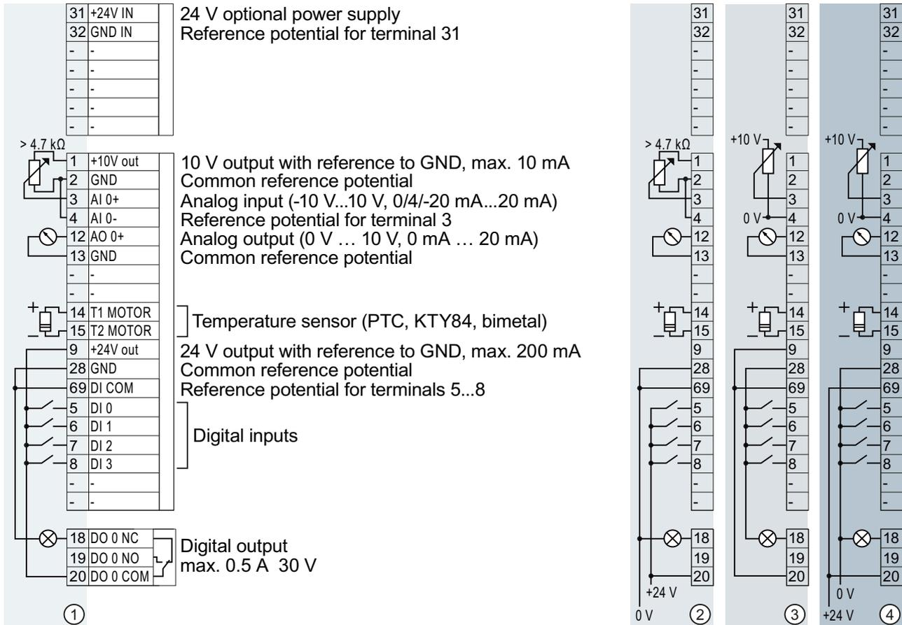
You may use the internal 10V power supply or an external voltage source for the analog input.
