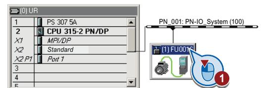
Open by double-clicking on slot 0 in the station window (2) the properties window for the network settings of the converter and activate there in the parameter (3) tab as shown the standard alarms (4).
