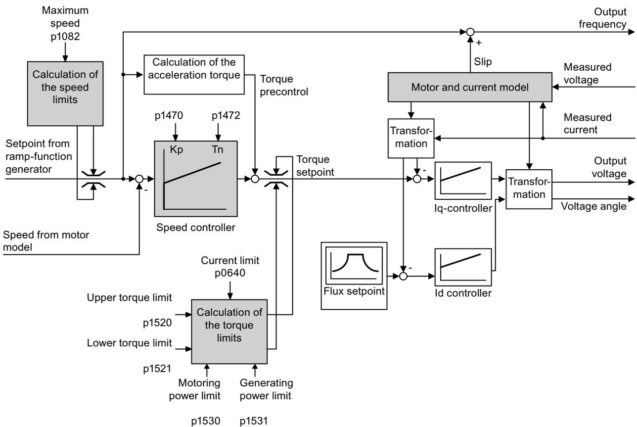
Figure 8-20 Simplified function diagram of sensorless vector control
