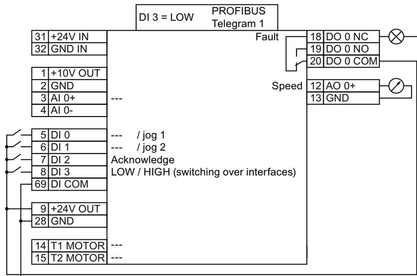
Figure 5-3 Wiring example to use the factory settings
