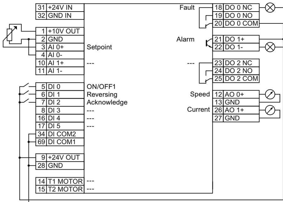
Figure 5-4 Wiring example to use the factory settings
