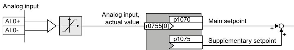
Figure 8-12 Example: Analog input 0 as setpoint source
