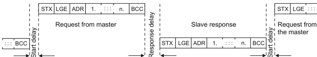
Figure 7-15 Start delay and response delay
