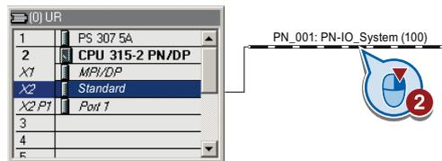
Open the properties window of the converter (⑤) and enter a unique and descriptive device name for the converter. You will also find the proposed IP address in this screen form. If required, you can change the IP address via "Properties".
