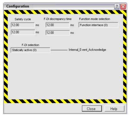
Figure 8-16 Configuring safety terminals
