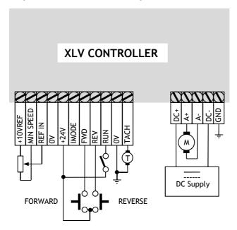
Note that the switches for forward and reverse running do not need to be latching as this function is within the controller.
