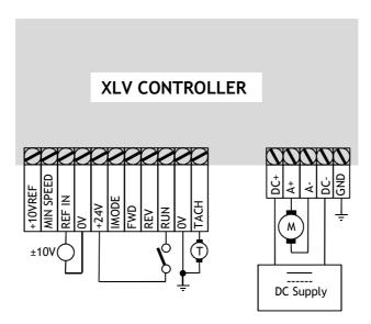
This configuration would typically be used when an external controller (e.g a positioning system) provides the speed reference.
