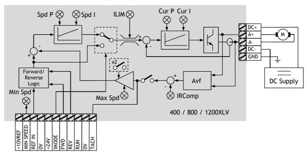
The RUN switch must be connected to +24V for the controller to operate. This is a NON-LATCHING input.
