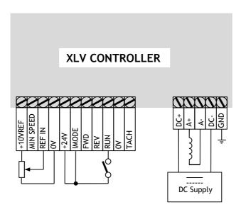
If operating a motor in this configuration, include measures to limit motor speed under light-load conditions.
