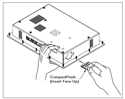
**Note:** Do not remove or insert the CompactFlash card while power is applied to the unit. Refer to the "Front Panel LEDs" section of this document for more information.
