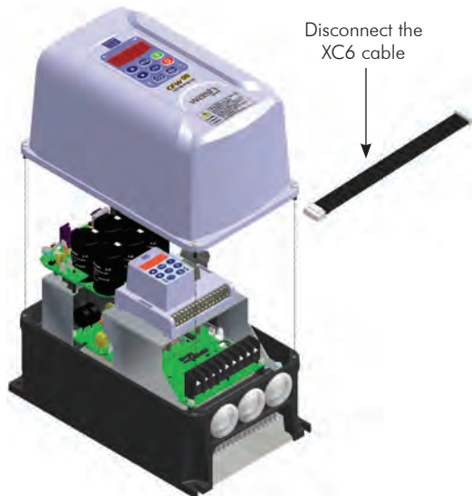
Figure 4.1 - Instructions for the XC6 interconnection cable removal
