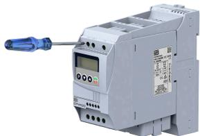
(d) Tighten the screws of the supply terminal of the CFW100 (Torque: 0.6 N/m)
