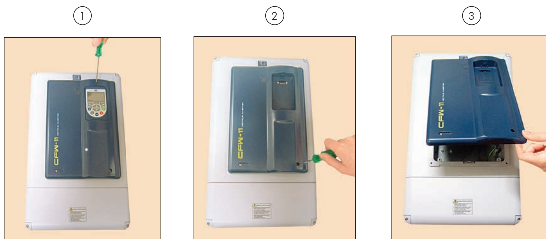
Figure 3.6 - HMI and control rack cover removal
