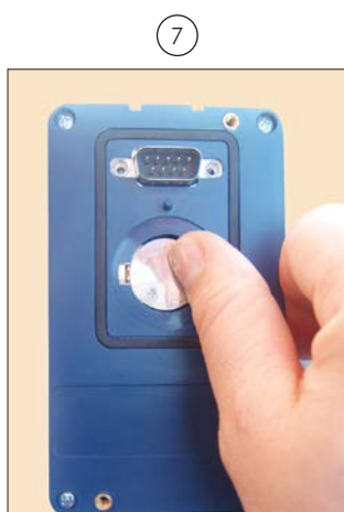
Press the battery for its insertion
