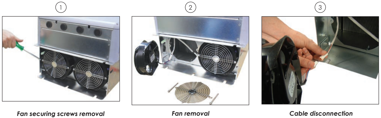
Figure 6.1 - Removal of the heatsink fans
