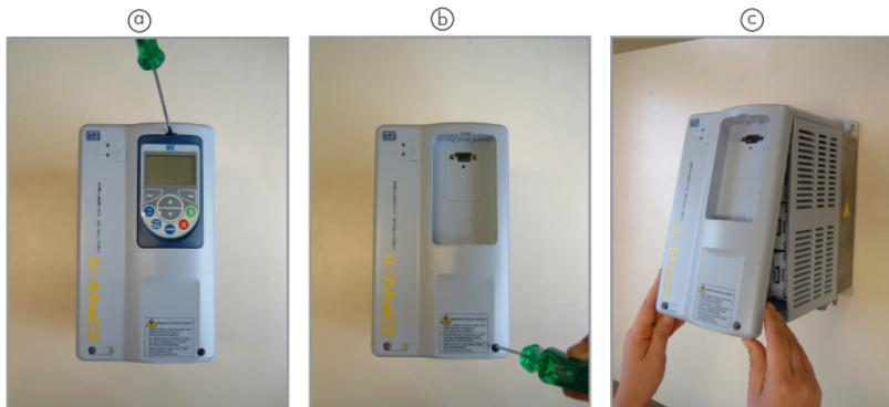
Figure 2: Removal of front cover
