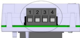
**Table 2:** Connector XC7 pins for RS-485 interface
