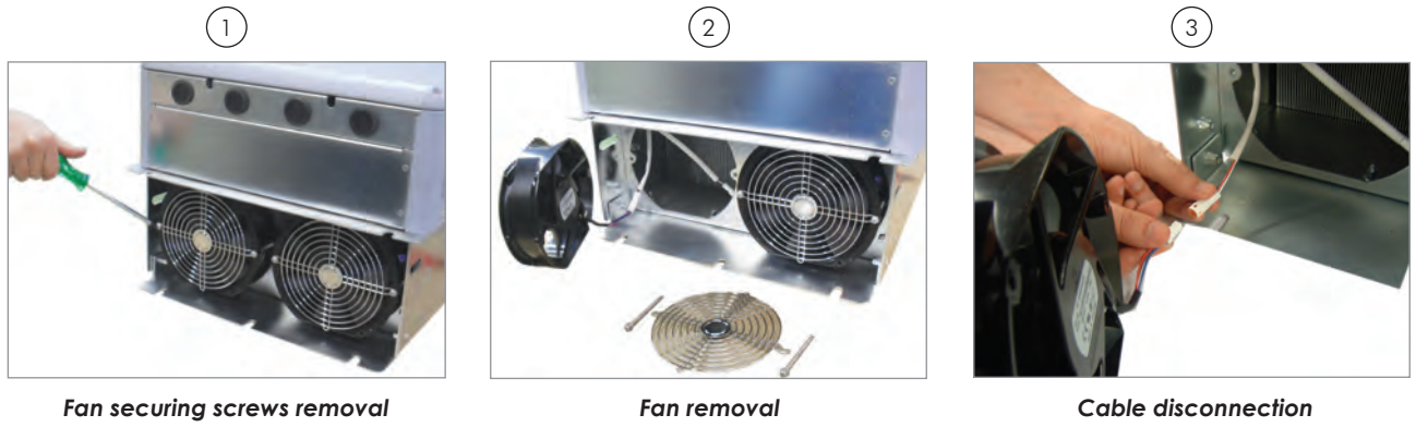
Figure 6.1 - Removal of the heatsink fans
