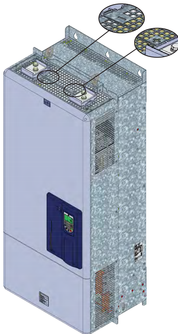
(d) Frame size G DC connection terminals (In models with special DC hardware, the R/L1, S/L2 and T/L3 terminals are not internally connected in this version)
