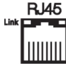
Besides the control connections, the module has a connector for Ethernet interface, which follows the 100 Base-TX Fast Ethernet standard.
