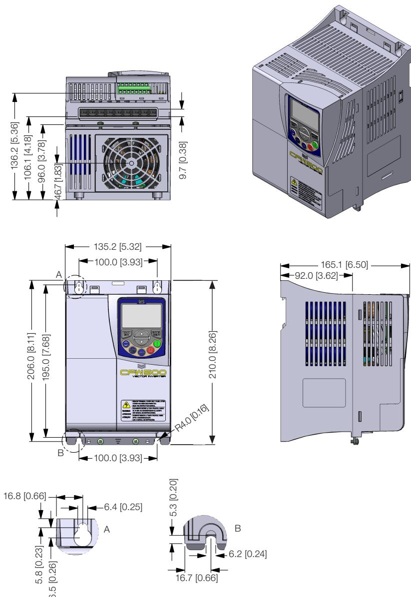
**Figure B.7:** Inverter dimensions in mm [in] - frame size C
