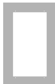
(c) Flange mounting - standard inverter (Only frame sizes F, G)
