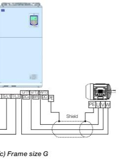
Figure 4: (a) to (c) Power and grounding connections
