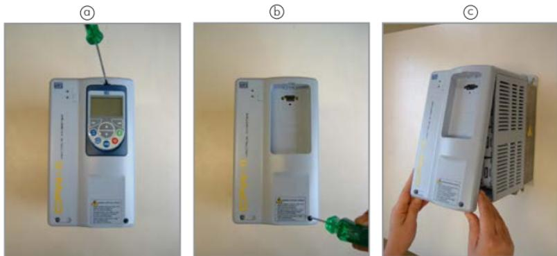
Figure 2: Removal of front cover
