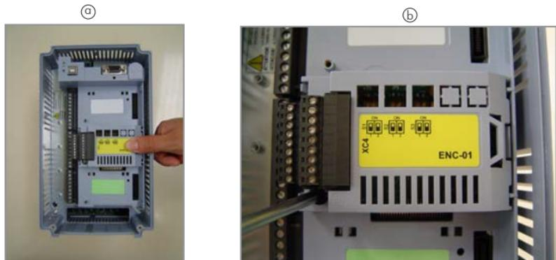
Figure 3: Installation of optional module into slot
