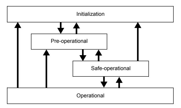
The adapter module enters the Initialization (INIT) state directly after start-up. After this, the adapter module can be switched to the Pre-operational (PREOP) state. In the PREOP state the EtherCAT mailbox communication is allowed and CoE objects can be accessed by SDOs.
