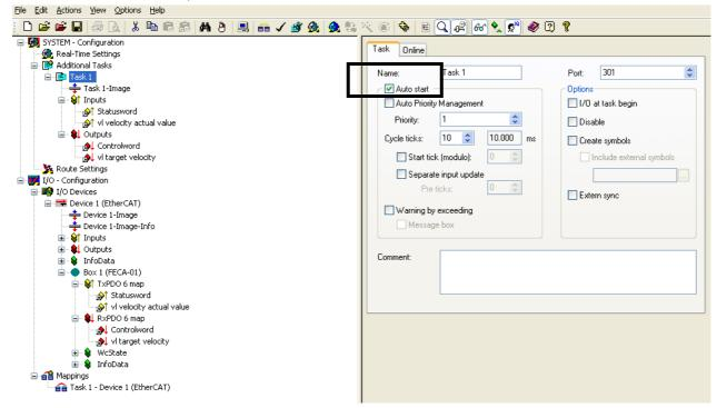
11. Change the TwinCAT configuration state using the buttons shown below. For example, take FECA-01 and the drive into the OPERATIONAL mode.
