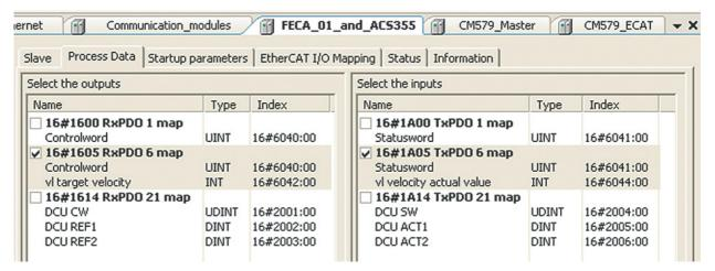
On the EtherCAT I/O Mapping tab, type names for the variables that refer to the drive's signals in the PLC program.
