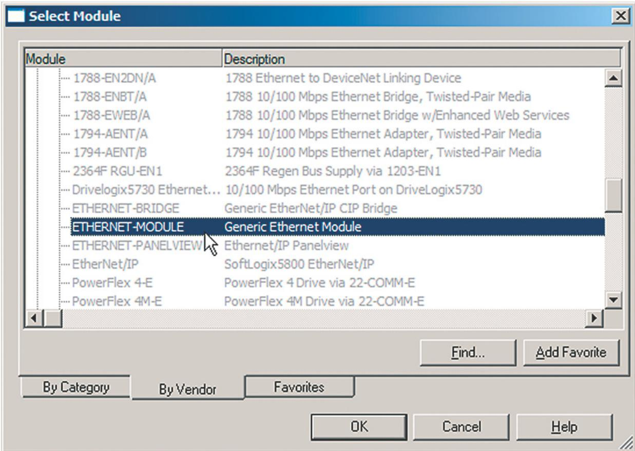
4. Select the input and output assembly instances and the PLC I/O memory size to be used. The table below shows the available combinations. The example below uses the ODVA AC/DC assembly instances 121 and 171.
