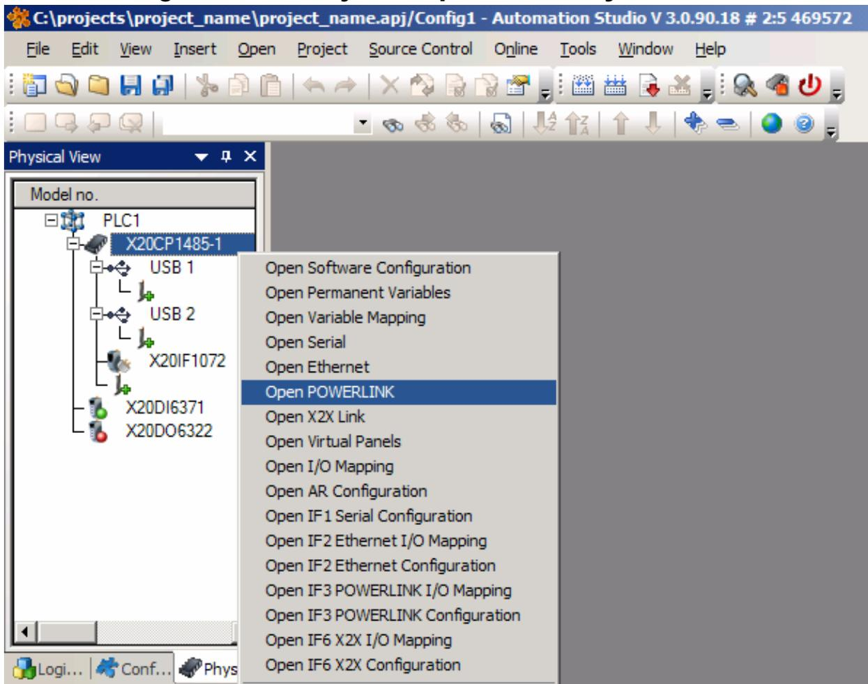
The POWERLINK window opens, displaying a list of the devices connected to the Powerlink interface (IF3) of the PLC.
