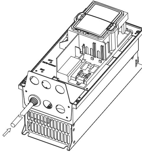
**Step 6:** Fasten the rubber grommet and cable with a self-locking cable tie.
