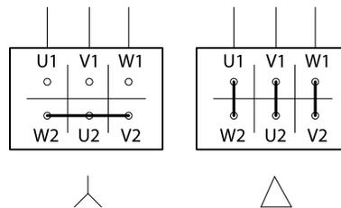
The three-phase motor with the rating plate based on **Figure 15**, can be run in a star or delta connection. The operational characteristic curve is determined by the ratio of motor voltage and motor frequency, in this case.
