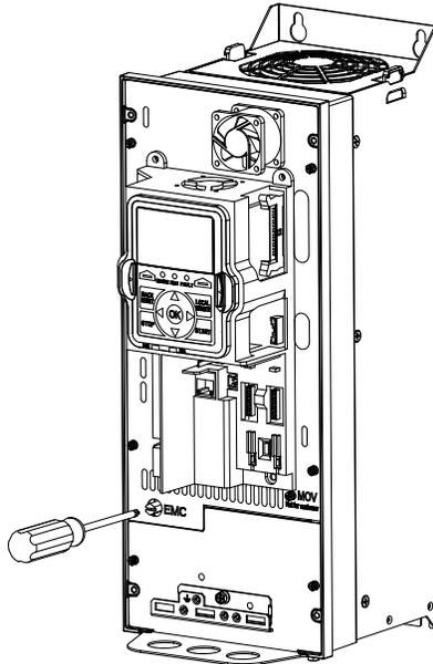
**Figure 38. Locations of EMC and MOV Screws for Frame 2 and Frame 4**
