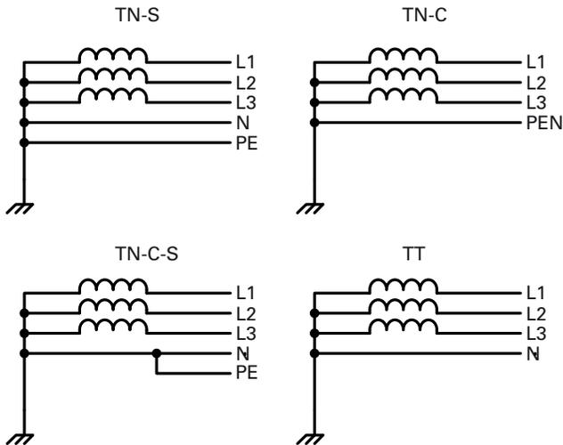
The frequency inverter can be applied to all types of power networks above. If multiple frequency inverters with single-phase supplies are to be connected, a symmetrical distribution to the three external conductors shall be taken into account. In addition, the total current of all single-phase consumers is not to cause an overload of the neutral conductor (N-conductor).
