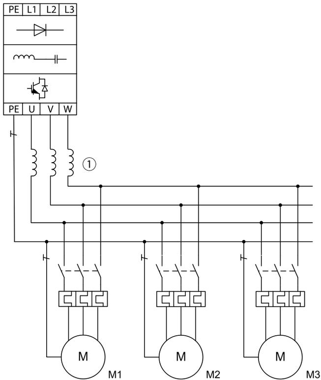
Connecting motors in parallel reduces the load resistance at the frequency inverter output. The total stator inductance is lower and the leakage capacity of the lines greater. As a result, the current distortion is greater than in a single-motor circuit. To reduce the current distortion, you should use motor reactors (see ① in **Figure 14**) in the output of the frequency inverter.
