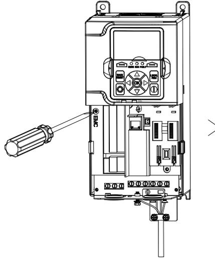
Figure 37. Locations of the EMC Screw in Frame 1 and Frame 3
