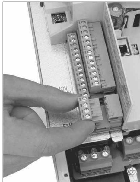
**Note:** For ease of access, the board terminals blocks can be unplugged for wiring.
