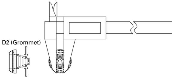
**Step 3:** Cut the rubber grommet at the selected diameter.
