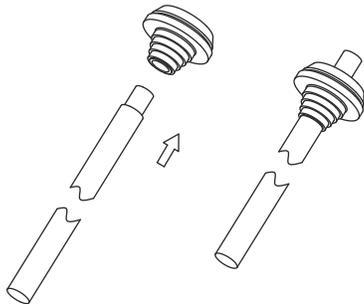
**Step 5:** Insert the rubber grommet into the conduit plate together with the cable.
