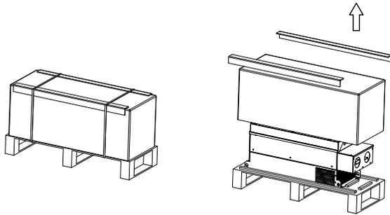
**Step 2:** Remove the four screws (used to fix the drive to the pallet) with an M8 or 3/8 inch wrench.
