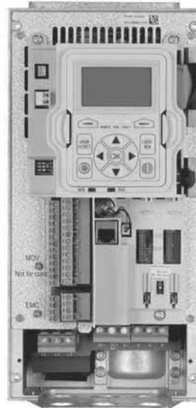
6. Wire power terminals (L1, L2, L3), motor terminal (U, V, W), and grounding terminals per **Figure 24**. It is recommended for power and motor leads to be in separate conduit
