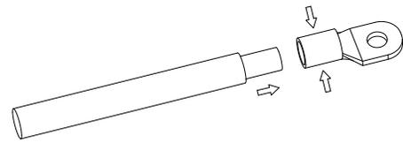
**Step 3:** Connect the power wire to the FR6 terminal block, lock the wire by a nut. Depending on the current level, one or two power wires can be connected to each pole of the terminal block.
