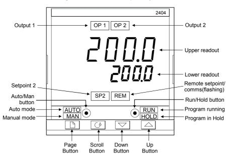
Figure 2-2 Model 2404 front panel layout
