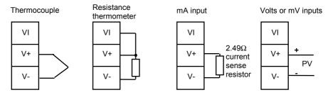
Fig 1-7 Sensor input connections
