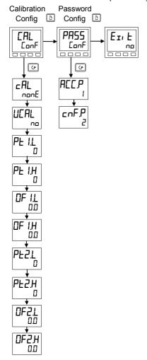
Fig 6.1c Navigation Diagram (Part C)
