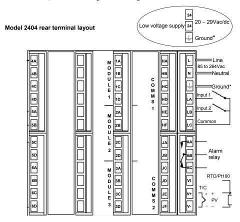
Figure 1-6 Rear terminal layout - Model 2404
