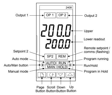
Figure 2-1 Model 2408 front panel layout
