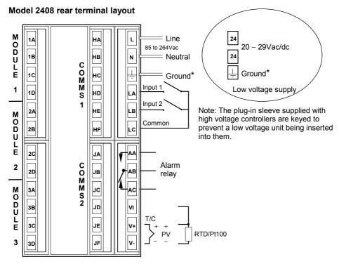
Figure 1-5 Rear terminal layout - Model 2408
