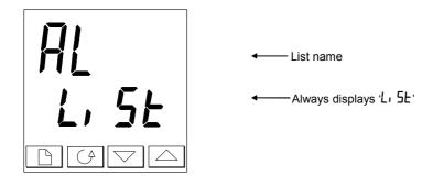
Figure 2-5 Typical list header display
