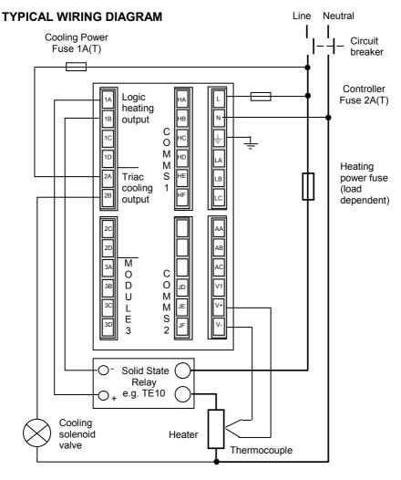
Fig 1-10 Typical wiring diagram, Model 2408 Controller
