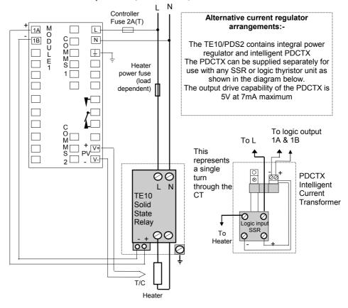
Figure D.1 Connections for Mode 1 & 2
