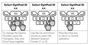
**NOTE** Once the User has set the Optipad as Device Number 2, Optistore or OptiTools software cannot be used on the same drive network. The Optipad Device Address should only be changed to 2 if 2 Optipad units are connected on a network. An Optipad with Device Number 1 must always be present for the network to function correctly.
