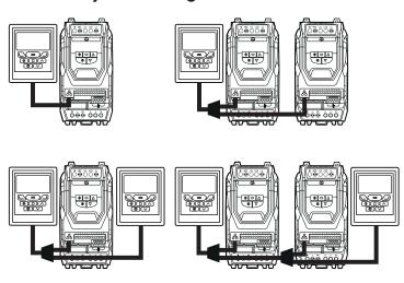
Different drive models can be used on the same Optipad network provided a unique communications address is assigned to each.
