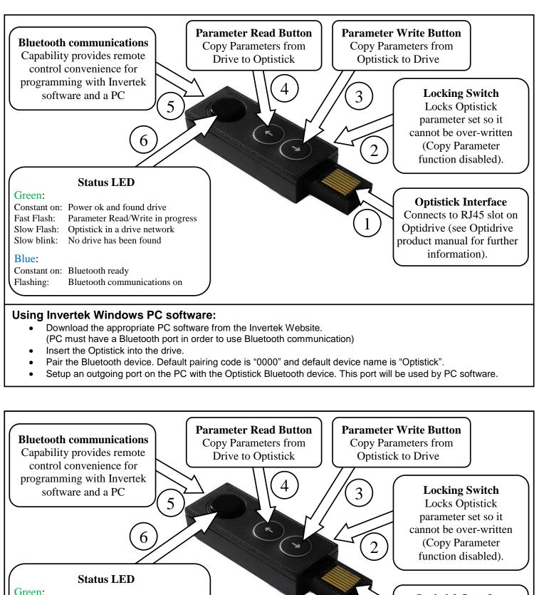
**Optistick Interface** Connects to RJ45 slot on Optidrive (see Optidrive product manual for further information).
