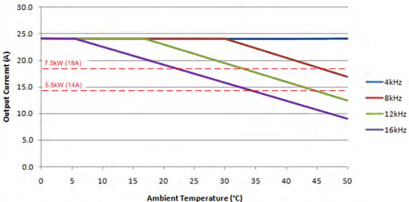
**5.6.2. 5.5kW and 7.5kW, IP66****ODP-2, Size 3, 400V, 7.5kW, IP66 Drive
