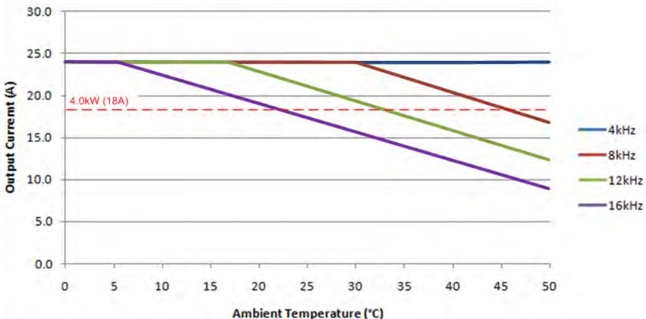
**5.5.2. 4.0kW, IP66****ODP-2, Size 3, 230V, 4.0kW, IP66 Drive
