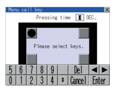
When setting 1 point, specify the time to switch to the utility in case of keeping pressing the key position.
