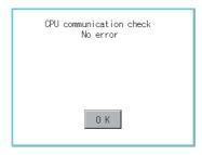
When the connecting target confirmation communication ends, its result is notified by dialog box. If the connecting target confirmation communication ends normally, the dialog box notifying of the normal termination mentioned left is displayed. Touching [OK] button after confirming the result returns to [I/O check].
