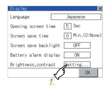
Touching the setting items displays the brightness contrast adjustment screen.
