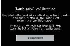
5. Touching the button displayed on the upper right returns the screen to the previous screen. When the precise touch could not be made, touch the [Readjustment] button to make the setting from again.
