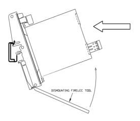
Dismounting of the unit on the rail DIN Push in the direction of the arrow
