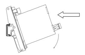
Mounting of the unit on the rail DIN
