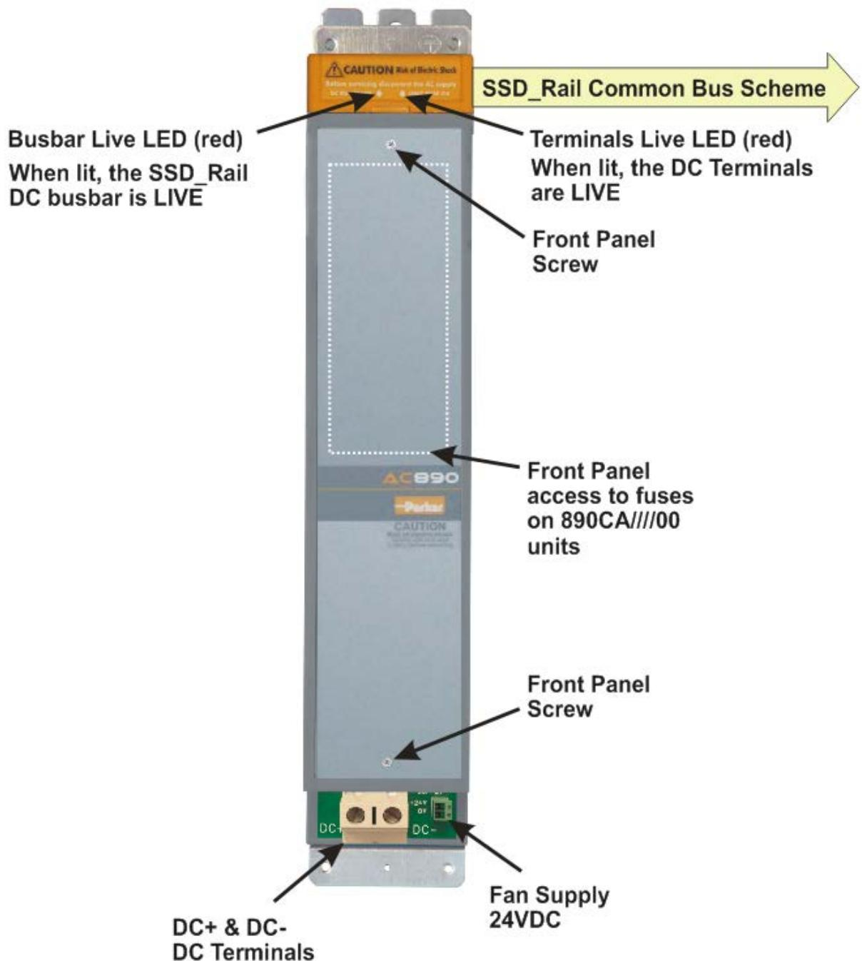
**IMPORTANT:** If only one LED is lit, an internal fuse has blown. Refer to page 14.
