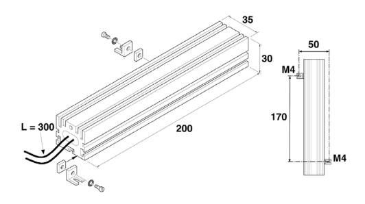
Overall Dimensions, Resistor 350W - IP55
