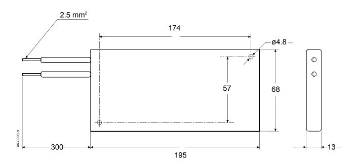
Overall Dimensions, Resistor 550W - IP55
