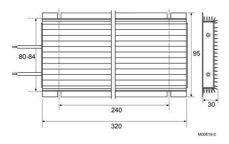
Overall Dimensions, Resistor 1100W – IP55
