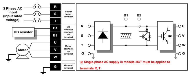
Power terminal wiring (11.0 ~ 22.0kW)
