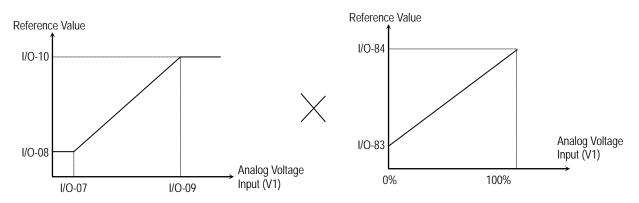
$$FBK \ display = \left( \left( \frac{I10 - I8}{I9 - I7} \right) \times \left( Input \ Voltage - I7 \right) + I8 \right) \times \frac{(I90 - I89)}{MaxFreq} + I89 \quad when \ feedback \ is \ from \ V1 = I89 + I89 = I8$$
