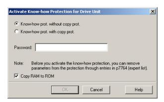
3. In this screen form, press the "Copy RAM to ROM" button. This means that you save your settings so that they are protected against power failure.
