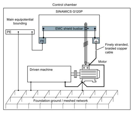
Figure 4-8 Additional high-frequency bonding of the drive system
