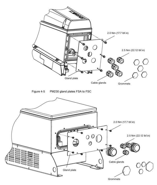
Figure 4-6 PM230 gland plates FSD to FSF
