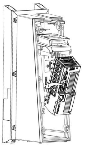
Due to the PM230 having either a cover to remove or a door to be opened to access the actual PM the fitting of the CU and the removal of the CU slightly differs; the complete fitting and removal instructions are given below.
