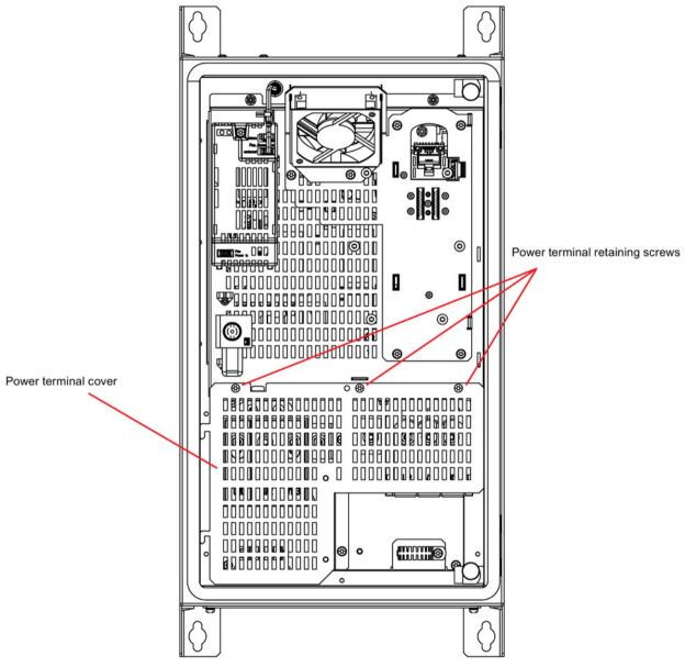
Figure 4-2 SINAMICS PM230 FSD to FSF Terminal Cover
