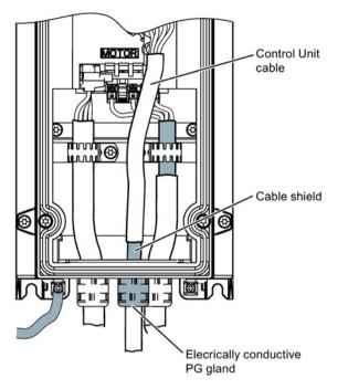
Figure 4-10 Control Unit cable shielding, FSA ... FSC
