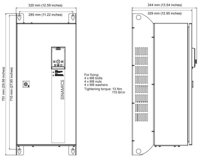
Figure 3-5 Dimensions and drill pattern, PM230 FSE (37.0 - 45.0 kW)
