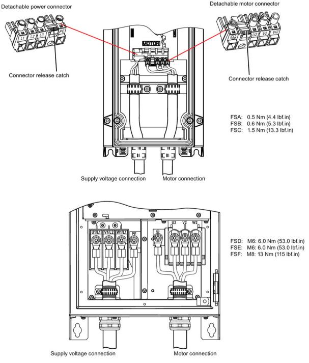
Figure 4-3 Power and motor terminal layout for FSA ... FSF
