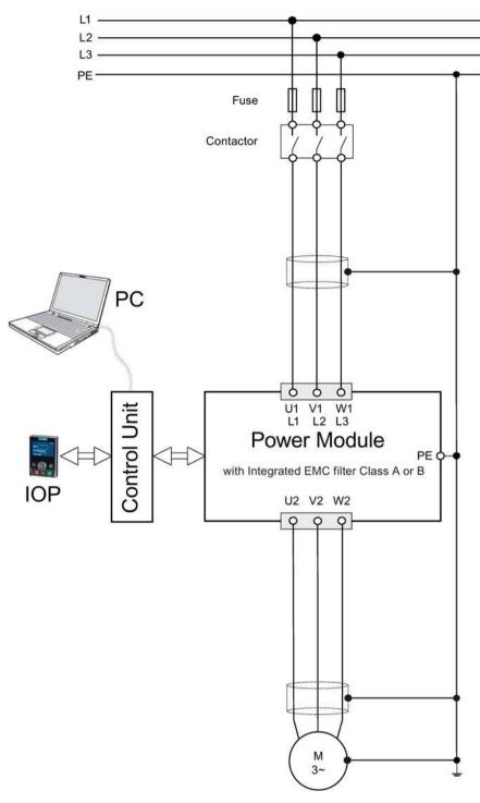
Figure 1-3 Block diagram PM230
