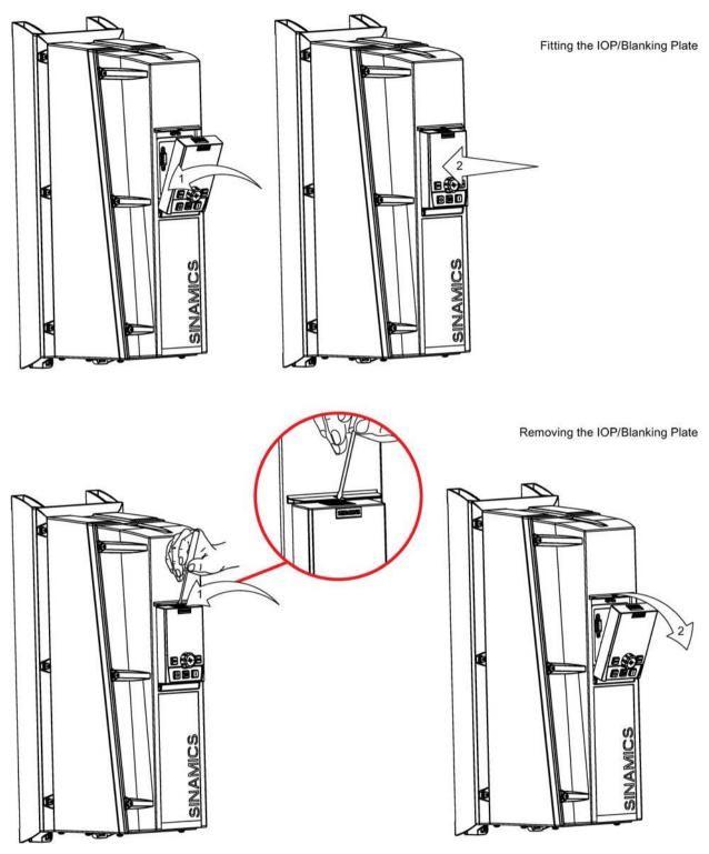
Figure 3-11 Fitting the IOP and blanking plate
