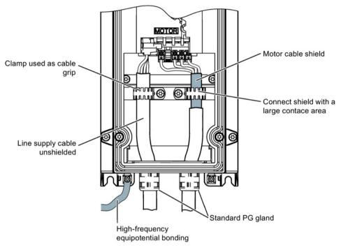
Figure 4-9 Power Module shielding, FSA ... FSC
