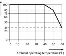
Figure 6-2 Current derating for temperature PM230 FSA ... FSF
