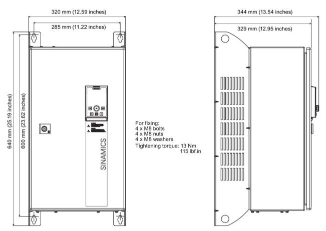
Figure 3-4 Dimensions and drill pattern, PM230 FSD (22.0 - 30.0 kW)
