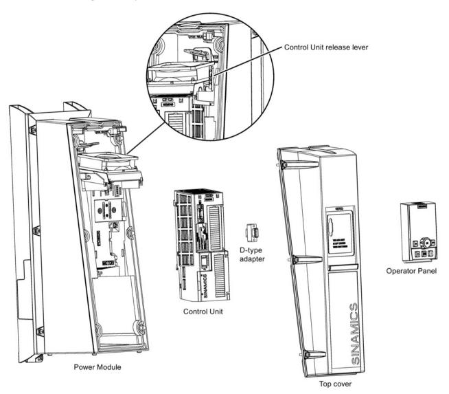
Figure 3-8 Fitting CU to PM230 FSA to FSC
