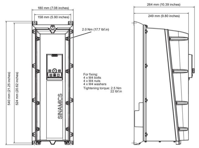
Figure 3-2 Dimensions and drill pattern, PM230 FSB (4.0 - 7.5 kW)
