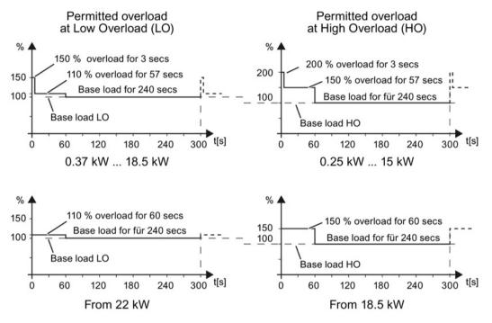
Figure 6-1 Duty cycles, "High Overload" and "Low Overload"
