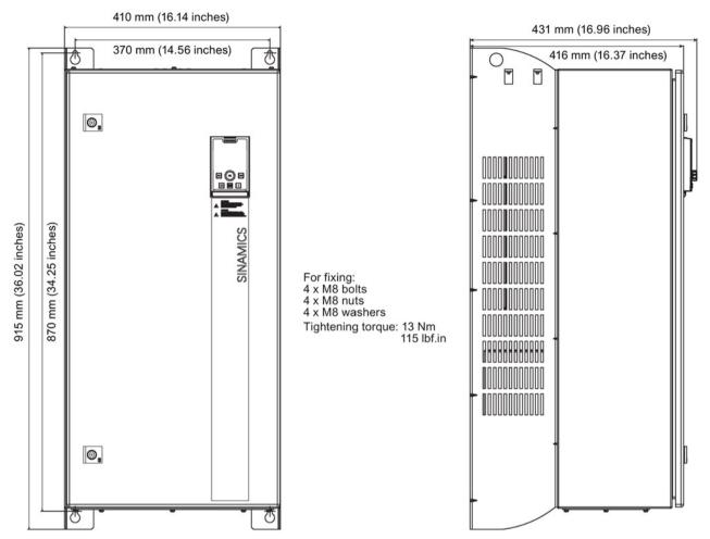
Figure 3-6 Dimensions and drill pattern, PM230 FSF (55.0 - 90.0 kW)
