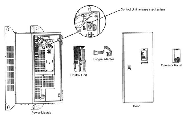
Figure 3-10 Fitting CU to PM230 FSD to FSF
