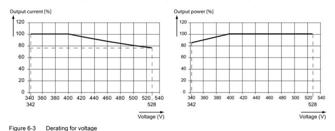
The figures below show the derating required according to voltage
