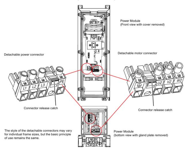
Figure 4-1 SINAMICS PM230 FSA to FSC power connections
