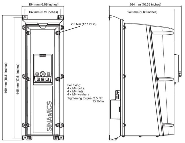
Figure 3-1 Dimensions and drill pattern, PM230 FSA (0.37 - 3.0 kW)
