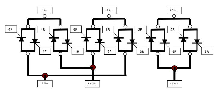
When 4 quadrant mode is selected the R pulses allow firing of a parallel bridge which introduces phase rotation at the output.
