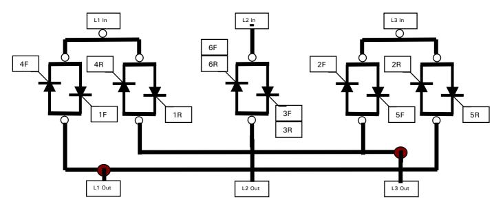
This 4 quadrant configuration saves on 2 thyristors. The 6F and 6R gate ouputs must be tied together and used to fire the gate as shown, in the usual way. Similarly the 3F and 3R gate driver outputs must be tied together and used to fire the other gate as shown, in the usual way. The gate outputs are able to be linked because they are open collector.
