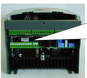
b) 2 way switch X (pole 2), FIRING (pole 1) 2) = X ON = 0, OFF = 1 (back) 1) = FIRING ON = 0, OFF = 1 (front)
