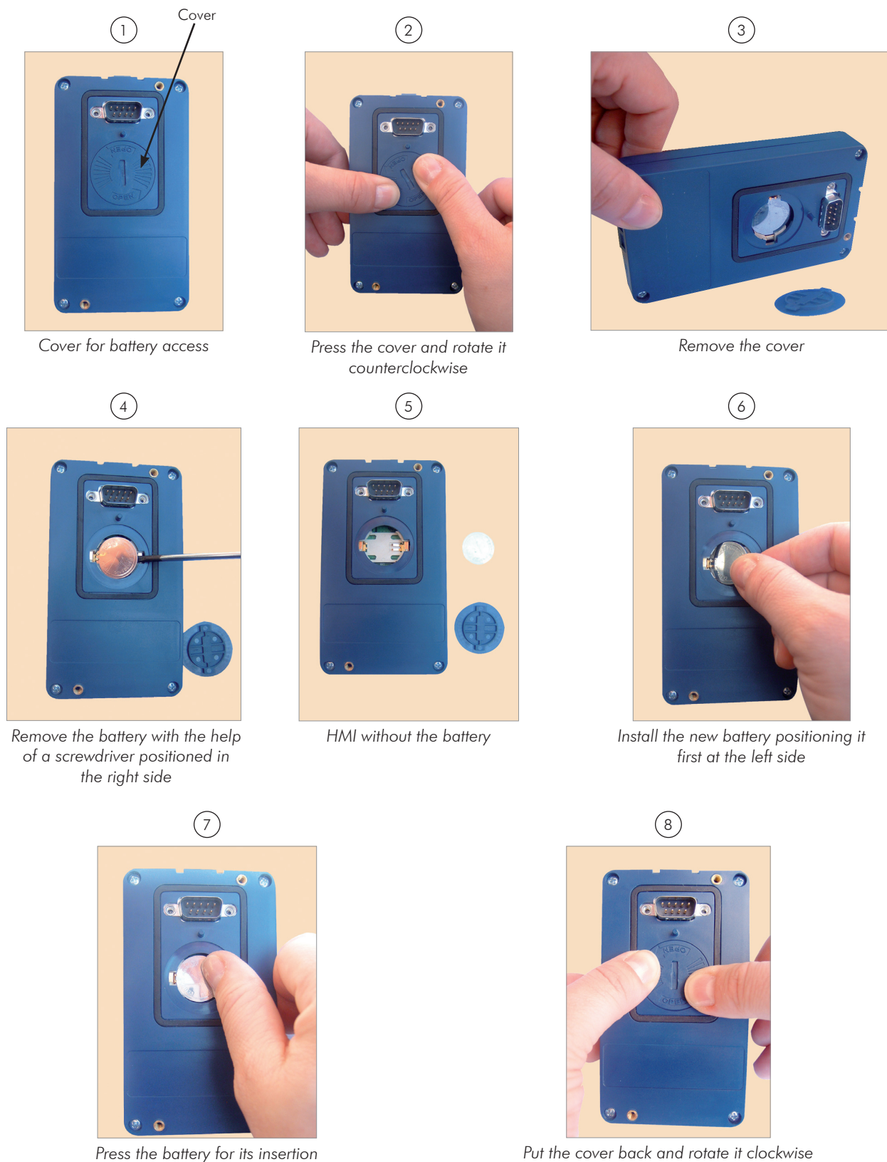
Figure 4.2 - HMI battery replacement
