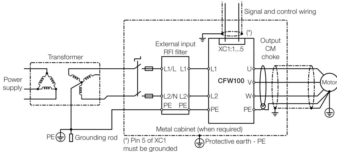
**Figure 3.4:** Connection of the RFI filter - general conditions
