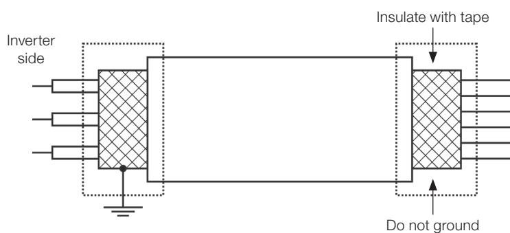
**Figure 3.3:** Shield connection
