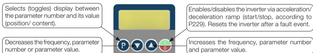
Figure 4.1: HMI keys
