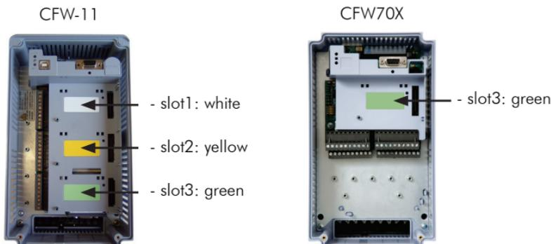
Figure 1: Identification of slots for accessories
