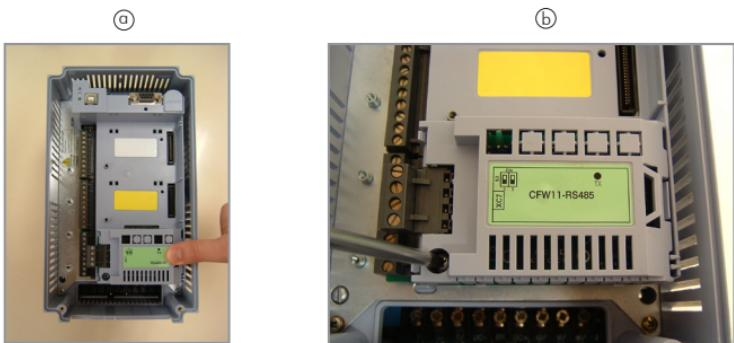
Figure 3: Installation of the accessory into slot
