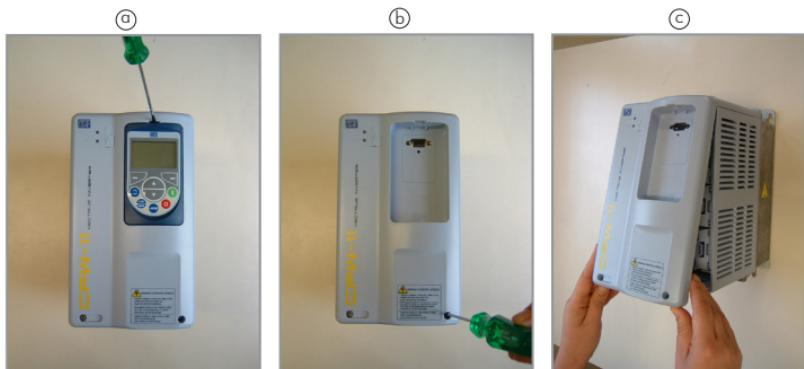
Figure 2: Removal of front cover
