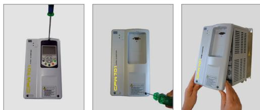
Access to the control and power terminal strips
