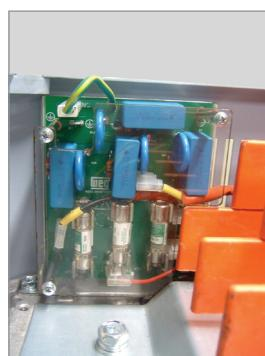
Procedure for disconnecting the RFI filter and the MOV connected to the ground – necessary for using the inverter in IT or corner-grounded delta networks
