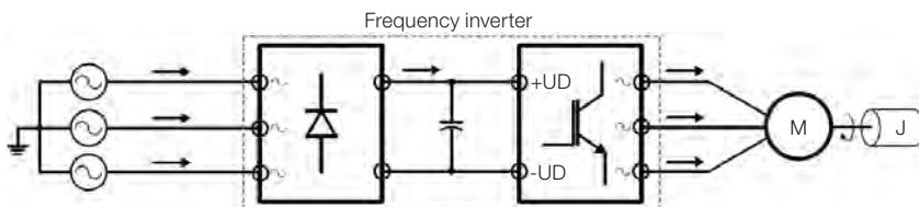
Figure 2.1: Motorization step
