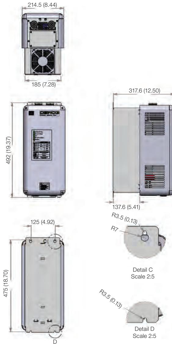
Figure 7.1: Dimensions of the DBW03 in mm (in)
