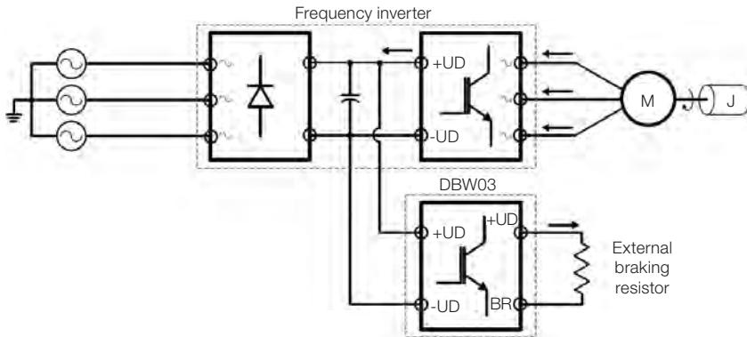
Figure 2.2: Braking step
