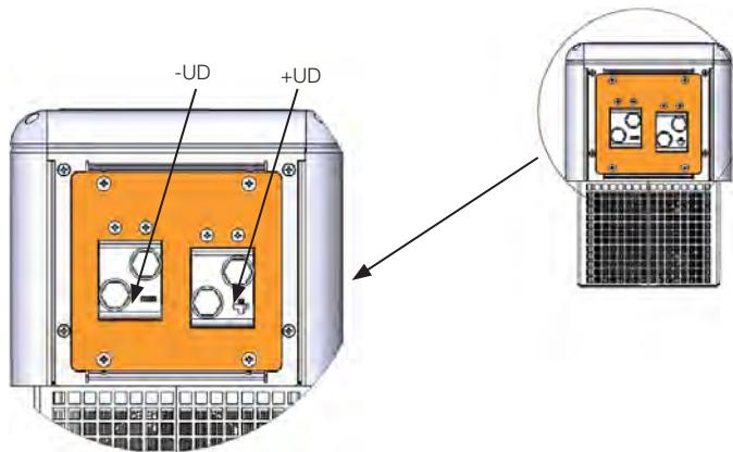
*Figure 3.3: Input connections +UD and -UD*
