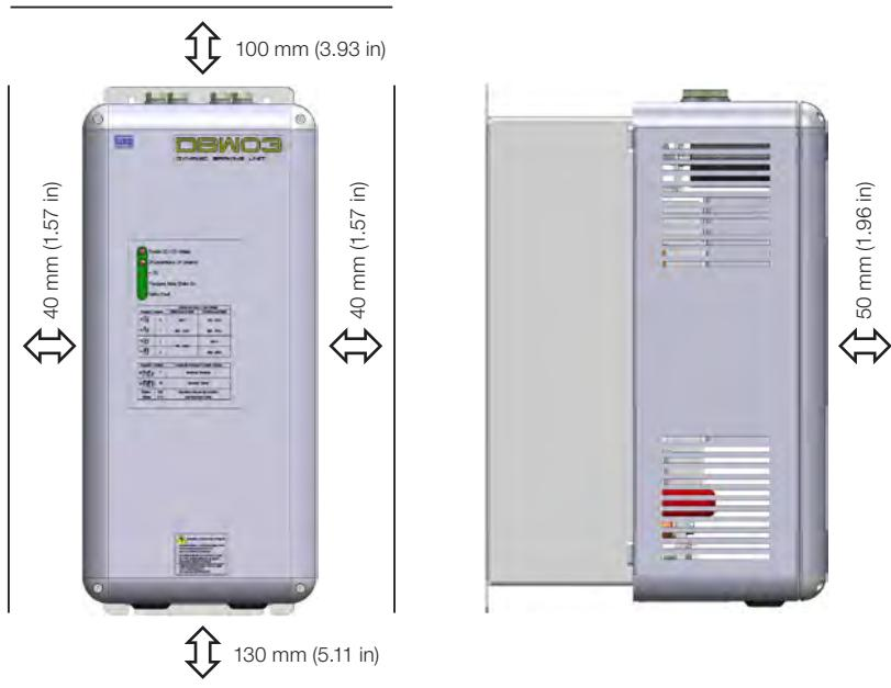
**Figure 3.1:** Ventilation clearances
