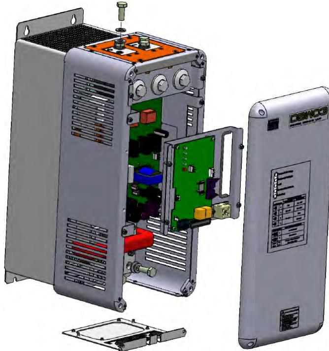
Figure 2.4: Main components of the DBW03 braking module
