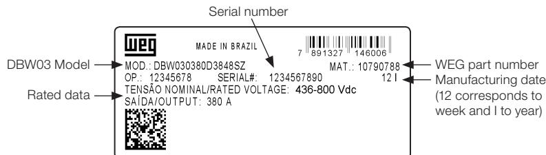
Figure 2.5: Example of identification label of the DBW03
