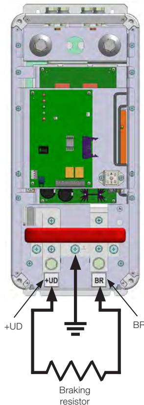
**Figure 3.4:** Connections of the grounding and braking resistor
