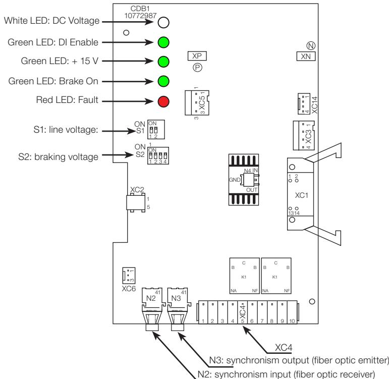
**Figure 3.7:** Connection points of the CDB1 board
