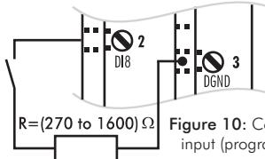
Figure 10: Configuration of DI8 to be used as a digital input (program every function at P270 excepting 16)
