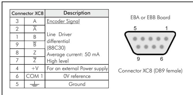
Figure 17: Output encoder signals connection and configuration
