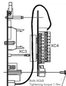
Figure 3: Bolt insertion
