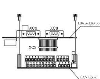
Figure 1: XC3 connector insertion
