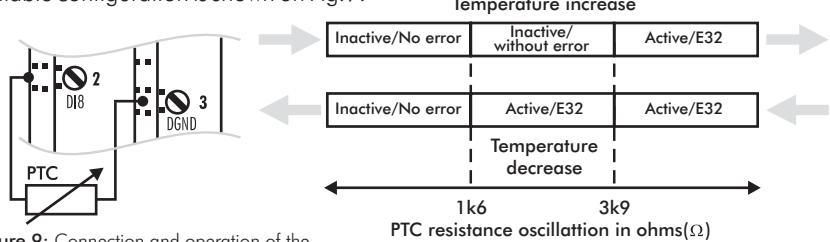
Figure 9: Connection and operation of the digital input DI8 with the motor thermistor function
