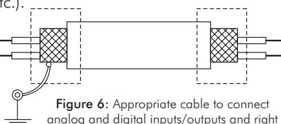
Figure 6: Appropriate cable to connect analog and digital inputs/outputs and right shield connection
